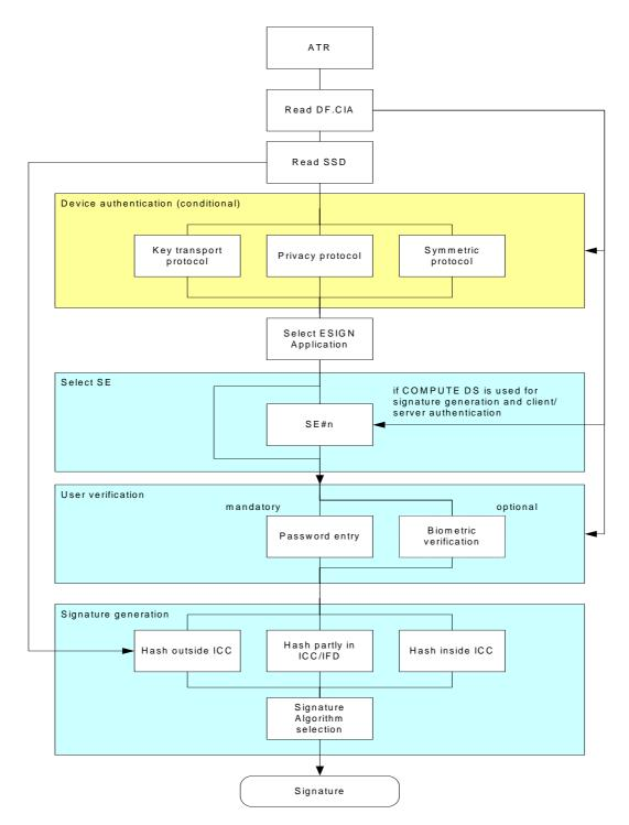
Figure C-1. Flow of selectable options for signature generation
