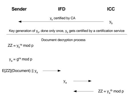
Figure 7-4. DH key exchange acc. to RFC 2631
