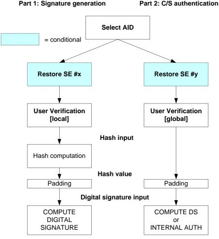
Figure 6-3. Comparison of operations in the ICC for signature creation versus C/S auth.
