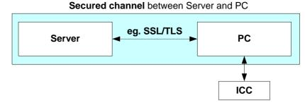
Figure 6-1. Example of client/server authentication
