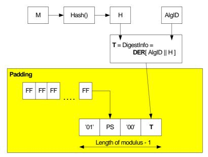
Figure 6-2. PKCS encoding of message M
